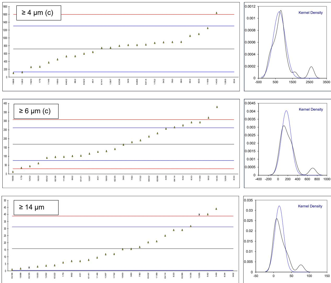
Determination of Level of Contamination acc. to ISO4406 scale on sample #21215; results in scale number
