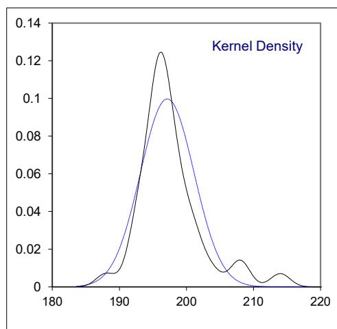
Determination of Kinematic Viscosity at 40°C on sample #21215; results in mm<sup>2</sup>/s
