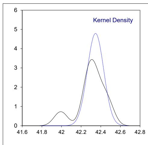
Determination of Kinematic Viscosity Stabinger at 100°C on sample #21215; results in mm<sup>2</sup>/s
