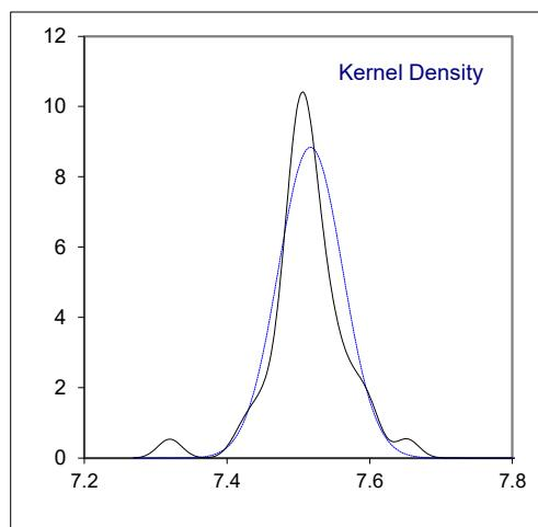
Determination of Kinematic Viscosity Stabinger at 40°C on sample #21215; results in mm<sup>2</sup>/s
